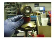
When installing the shock on the car for the first time, the REB adjuster should be set at minus 24 clicks, from "Full Stiff". This is a good place to start, "mid range".
