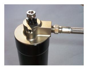
When installing the shock or strut on the car for the first time, the LSC adjuster (the small knurled knob) should be set at minus 15 clicks from "Full Stiff" and the HSC adjuster (the ½" hex knob) should be set at 6 clicks from "Full Soft". This is a good place to start, "mid range".
