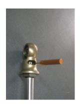
When installing the shock or strut on the car for the first time, the REB adjuster should be set at minus 12 sweeps from "Full Stiff". This is a good place to start, "mid range".
