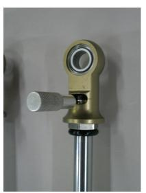
When adjusting the Rebound adjuster the Compression Bleed adjuster will spin with rebound adjustment. Do not worry about it, it is supposed to, they are independent of each other and will not affect each other until you adjust each one.
