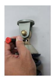
When installing the shock or strut on the car for the first time, the REB adjuster should be set at minus 12 sweeps from "Full Stiff". This is a good place to start, "mid range".
